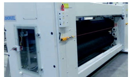
Pre-cylinder tacker for batt pre-consolidation
